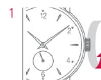
1 Rotate the crown carefully multiple times clockwise until you feel resistance.
